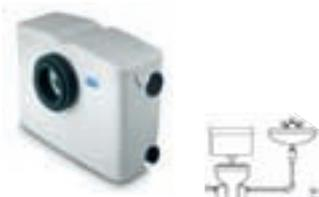
The Piranhamat 100-120 is designed for domestic wastewater removal from one WC located below the sewer backwash level or where sewage cannot flow by gravity into a sewer. It is also possible to connect one wash-hand basin, one shower and one bidet to the unit. The Piranhamat 100-120 is supplied plug-in ready with gas and odour tight tank and Piranha grinder pump.
