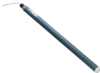
The KV is a conductive level switch, primarily used as overflow switch in sewage pumping pits. The KV can also be used in other applications where the conductivity of the media is between 25 and 750  $\mu\text{S}/\text{cm}$ .
