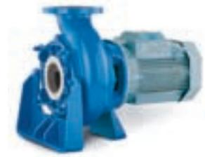
The dry installed sewage pump FR is developed for economic pumping of heavily polluted sewage and wastewater in municipal and industrial applications. The back-pull-out design utilizes standard electrical motors, making the pump service-friendly. Ample space inside the impeller and volute makes the pumps less prone to clogging. A double seal arrangement makes dry running possible. The units are supplied with vortex impellers or with the Contrablock system for reduction of clogging.
