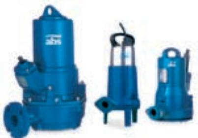
The Piranha range includes submersible sewage pumps with a shredding action cutting up the sewage into small particles. This allows for reliable discharge of domestic sewage under pressure using small discharge lines. It is suitable for sewage removal from houses, especially in rural areas where higher elevations must be overcome, or where only small diameter pipe work can be laid. The Piranha can also be used for heavily polluted wastewater.
