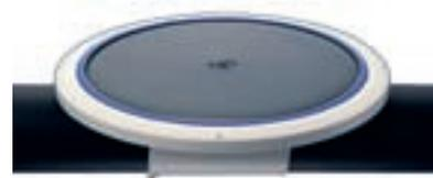
ABS Nopon disc diffuser system offers a number of alternative diffuser models (HKL, KKI, PIK, PRK, PRF, DS 20), which are easy to install and maintain. The diffusers have special features that improve the operation reliability and efficiency, such as the non-return valve available on all models and the sliding ring available on the latest version of ABS Nopon diffusers. High oxygen transfer efficiency combined with low pressure drops makes the ABS diffusers extremely effective.
