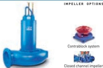
ABS submersible sewage pump AFP (ME4 & 5) is designed for larger applications pumping unscreened sewage in industrial and municipal applications. The pumps have high efficiency water pressure-tight encapsulated fully flood-proof motors in standard or explosion proof version supplied with the option of a closed loop cooling system. Suitable for both wet and dry installation.
