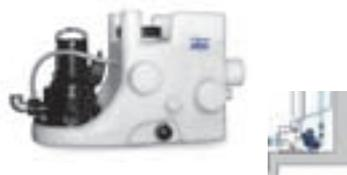
The Piranhamat 701 is a flood-proof lifting stations for automatic sewage removal from areas below the backwash level. This unit is fitted with one ABS Piranha submersible grinder pump suitable for pumping domestic wastewater. This range of lifting stations is ideal for locations where the diameter of the discharge line is restricted.
