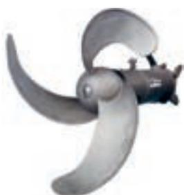
The ABS submersible mixer SB 1200 KA combines all the specific requirements of those treatment processes where the biofilm is bound on the surface of plastic carriers. The low tip speed in combination with a special designed propeller, prevent any negative effects on the carrier material during the mixing. The energy cost is reduced thanks to a unique drive unit design including a high efficient gear box.
