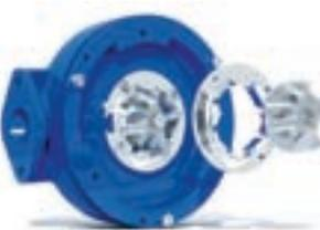
The ABS Piranha cutting system offers a unique concept in grinder pump design. Our cutter design features a lobed rotor cutter attached to a centrifugal impeller together with a stationary cutting element designed in a wave form. This causes an opening to be formed between the rotor and stationary cutter, which results in the huge number of 15,000 cuts per minute. The solids are sheared into particles as small as 1 mm, which allows them to be pumped through small bore pipes.
