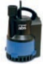
The Robusta has been designed for pumping clear and wastewater from house, garden or yard and can pump away even very low water levels. It is supplied with built-in level control and check valve. The pump and motor section form a pressure-tight encapsulated and fully flood-proof unit. The pump is suitable for manual or automatic operation.
