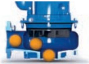
The ABS vortex impeller has been designed to maximise the size of solids handled, allowing all items found in wastewater to be passed without blocking the pump. The Vortex impeller is the natural choice when risk of blockage is high and lower efficiency can be accepted, for example storm water applications with low running hours. Other suitable applications are pumping liquids containing air, gas, coarse particles or items which can become trapped.
