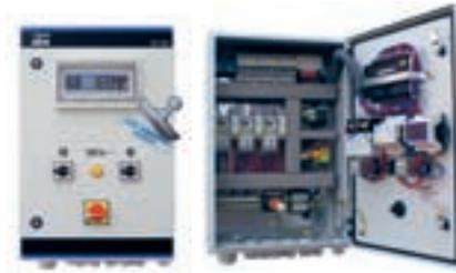
ABS Advanced Control Panels are providing a complete solution for a 2-pump pumping station. They are built around the PC 242 controller with advanced control and monitoring features. Two pumps in the power range of 1.5 to 22 kW can be controlled via DOL or built in soft starter, additionally a contactor for a sump mixer up to 5.5 kW is provided. They are designed according to EN 60204-1. A modem for data transfer to the ABS AquaWeb system can be fitted.
