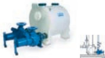
The Sanimat 1500 - 3700 is a flood-proof lifting station for automatic removal of domestic & commercial wastewater from areas below the backwash level. It is ideal for both new and renovated structures in large buildings; multi-family housing units, hotels, hospitals, etc. The Sanimat has a robust and corrosion resistant synthetic (PE) 140-350 litre collection tank with compact design and large storage capacity.
