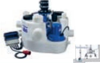
The Sanimat 1002 is a two pump version of the Sanimat 1000 designed for use in applications where the additional security of a standby pump is required. Robust synthetic (PE) 140 litre collection tank of compact design. Easy to transport.
