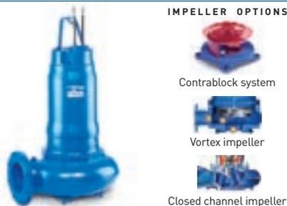
ABS submersible sewage pump AFP (ME3) is designed for reliable and economic pumping of unscreened sewage in industrial and municipal applications. The pumps have high efficiency water pressure-tight encapsulated fully flood-proof motors in standard or explosion proof version supplied with the option of a closed loop cooling system. Suitable for both wet and dry installation.
