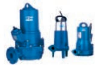
The Piranha range contains submersible wastewater pumps with a shredding action cutting up the domestic wastewater into small particles. This allows for reliable discharge of effluent under pressure using small diameter pipework.
