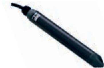
The HSR is a wastewater resistant, PVC encapsulated, 2-wire loop powered, submersible, hydrostatic level sensor. It is designed for level measurement in liquids like stormwater and wastewater in pump sumps. When connected in series with a DC power supply, the HSR gives a 4 to 20 mA output signal which is proportional to the level of the liquid.
