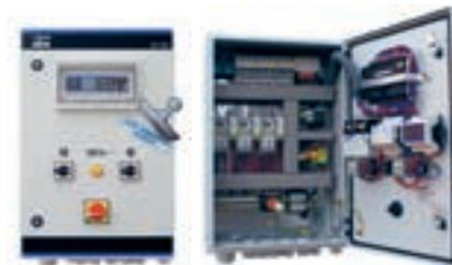
ABS advanced control panels provide a complete solution for a 2-pump pumping station. They are built around the PC 242 controller with advanced control and monitoring features. 2 pumps in the power range of 1.5 to 22 kW can be controlled via DOL or built in soft starter, additionally a contactor for a sump mixer up to 5.5 kW is provided.
