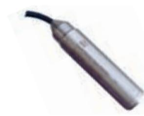
The HSC2 is a sewage water resistant, stainless steel encapsulated, submersible, hydrostatic level sensor of high accuracy. It is designed for level measurement in liquids like stormwater and sewage in pump sumps. The HSC2 loop powered level sensor gives a 4-20mA output signal which is proportional to the level of the liquid. Also available in Ex-version.
