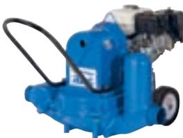
ABS engine driven diaphragm pumps are sturdy pumps for high solid content and shallow conditions. They are ideal for slow seepage applications with muddy water or sludge. The dry-running capability and self-priming function makes the diaphragm range reliable for keeping any area dry.
