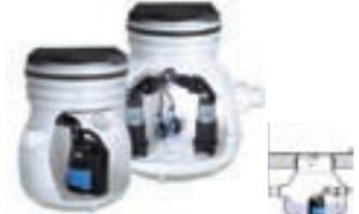
The Nirolift and Sanisett series provides simple and quick removal of faecal free wastewater from areas below the backwash level, suitable for installation either above or below ground. The tank is made from a robust corrosion-resistant synthetic material with optional odour control systems available. The wastewater pump is a standard Robusta or MF pump.
