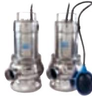
The ABS light drainage pump IP is a stainless steel pump for corrosive media with vortex hydraulics. It is suitable for pumping aggressive media with a high proportion of solid or fibrous matters. The IP is also ideal for dewatering of chemically contaminated wastewater, industrial effluent, and for use in agriculture. Level control switch is an option.
