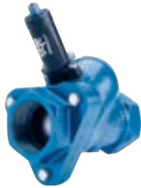
The ABS flushing valve is a programmable flushing valve for clean deposit-free sumps. Automatic sump cleaning avoids manual or mechanical de-sludging. By fitting the programmable flushing valve the pumped flow of the pump itself can be used to produce an intensive rinsing and flushing of the sump.
