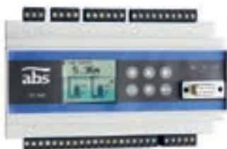
The PC 242 is a 2 pump controller designed mainly to be used in municipal wastewater pumping stations. It is has many advanced features to minimise the costs in the pumping station throughout the whole life cycle. The controller provides for various level measurement systems, current and power measurement, direct connection of motor monitoring devices and the control of a sump mixer. The unit can communicate with the ABS AquaWeb system via modem.
