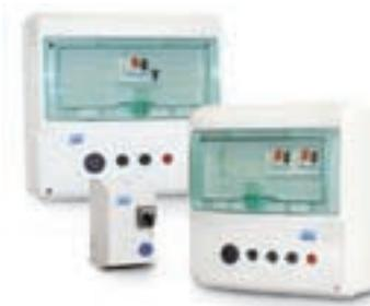
The ABS basic pump controller BPC is used for single and twin pumping stations up to 3 kW, single and three phase. With manual thermal protection reset. No Di seal monitoring. Suitable for lifting stations, sewage pumping stations and packaged pumping stations in accordance with EN 60204-1.
