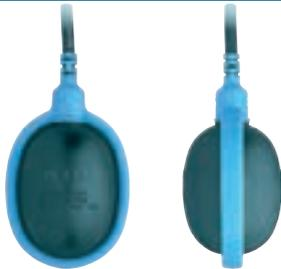
The ABS float switch can be used in liquids for control operations by using the liquid level. It is suitable for use in sewage. In the float switch a ball moves depending on the floating position and operates a high quality micro switch. The recessed rolling surface for the ball ensures trouble-free functioning even if the cable is twisted.
