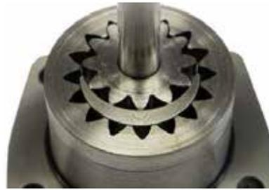
Internal gear pump
