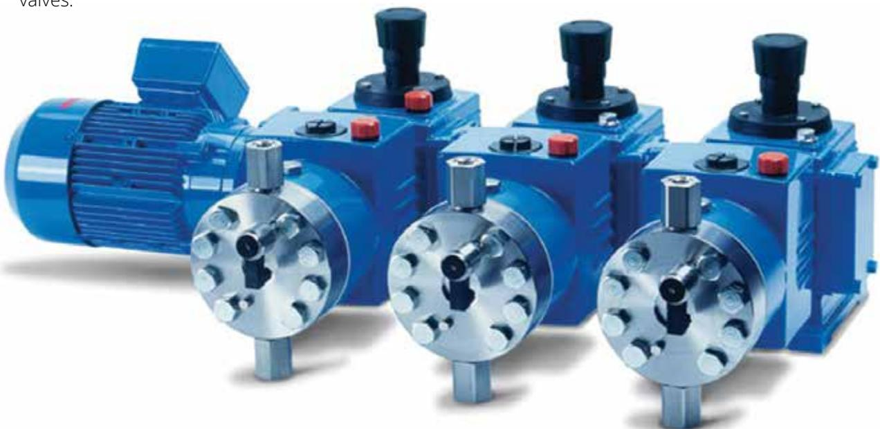
**Piston and Plunger Pumps** Both Piston and Plunger Pumps work with the linear motion displacing fluid inside of a cylinder. The difference is that the seal on the piston moves with the piston contacting the cylinder wall to create a seal. The plunger on a Plunger pump passes through a stationary seal and will generate higher pressure than piston pumps.
