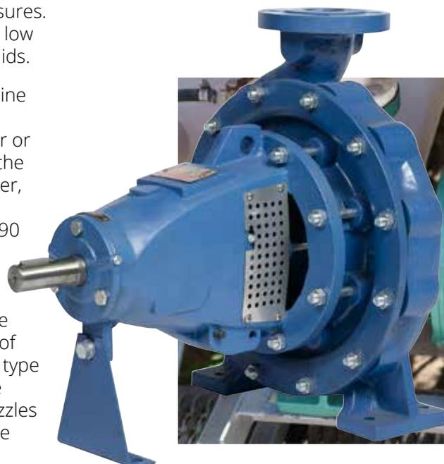
**Slurry** Pumps are the workhorses of the mining industry. They are robust pumps usually constructed from thick cast iron to withstand abrasive fluids mixed with solids like concrete, mud and other viscous, abrasive materials. The casing has a replaceable rubber coating or lining to protect the metal from damage. The impeller vanes are shorter to allow passage of stones and solids without damaging the system.
