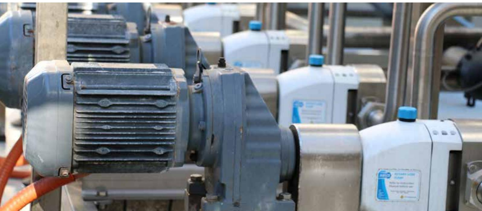
**Gear Pumps** Rotary Gear Pumps consist of at least one or two sets of rotating gears with intermeshing teeth. As the teeth separate, they create a partial vacuum which is filled by the fluid. When the gears continue to rotate, the fluid becomes trapped and carried around the casing to the discharge port of the pump. Gear pumps can be external or internal.
