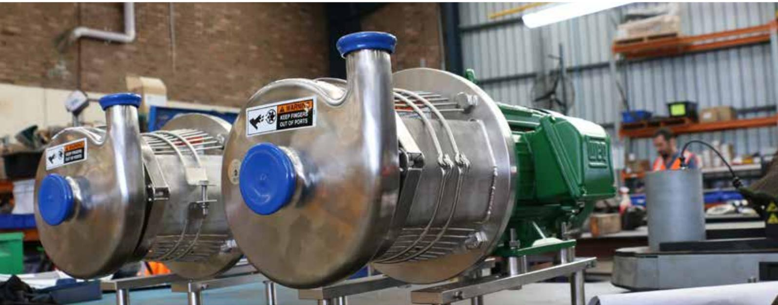
Pumps have strict tolerances and precise conditions under which they must operate to generate the Best Efficiency Point or BEP. Every pump has a chart showing the performance curves and how to attain the BEP. Pump manufacturers calculate performance curves with a pressure gauge and a flow meter connected to the discharge port to find the optimal configurations of piping, type of fluid and head. The discharge capacity can be calculated for any head.
