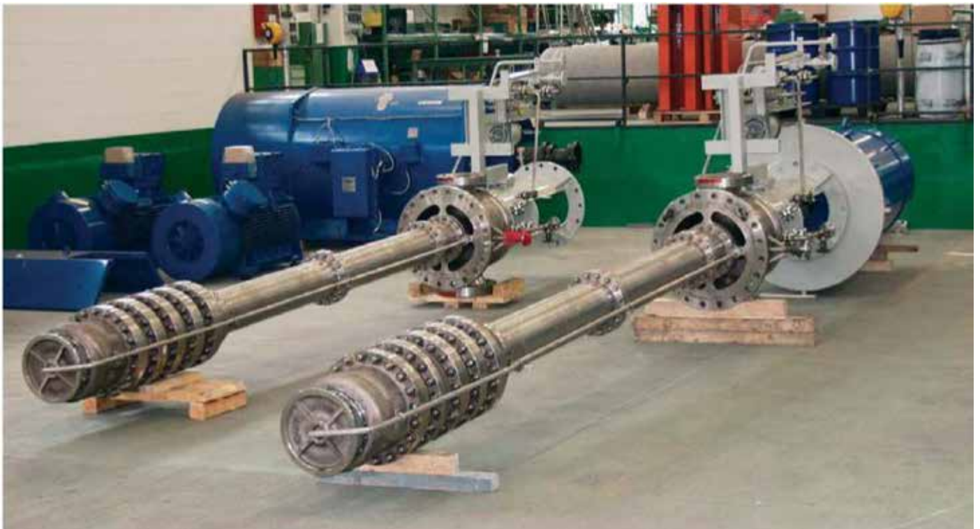
VBN pumps in Gabbioneta test room
