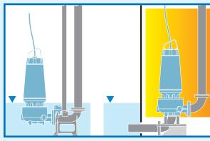
Continuous operation of the pump (S1 duty) is ensured even in dry and partially submerged working conditions or in high temperature locations.
