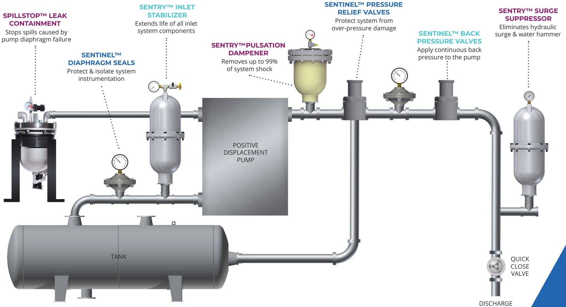
Installation of the pulsation dampener should be no more than ten pipe diameters from the pump's discharge. Additional pump system diagram featuring the Hybrid Valve™ configuration is available on page 29 of this guide.
