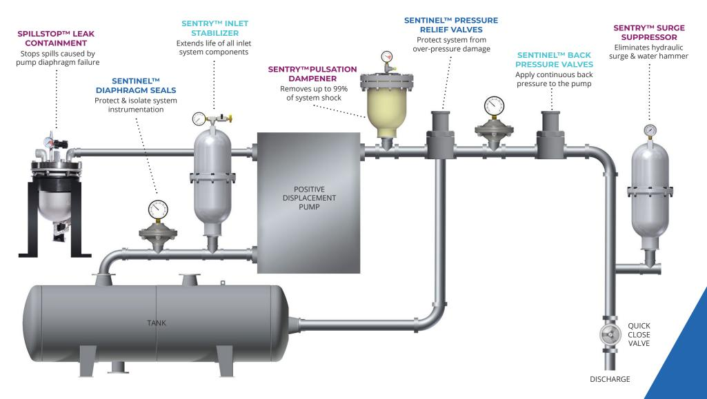
Installation of the pulsation dampener should be no more than ten pipe diameters from the pump's discharge. Additional pump system diagram featuring the Hybrid Valve™ configuration is available on page 29 of this guide.
