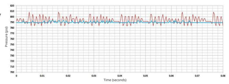
TRIPLEX PUMP with SENTRY XPA & XPH Dampener
