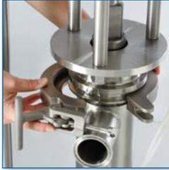
**All SaniForce Piston Pumps have Quick Knockdown Lower for Fast and Easy Cleaning!**
