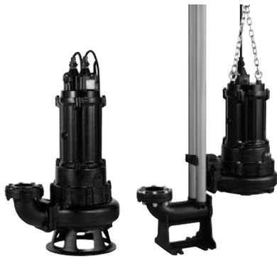
The C-series is a submersible cutter pump for sewage and wastewater, which is made of casting and equipped with cutting mechanism. Featuring a combination of impeller vane with brazed sintered tungsten carbide alloy edge and a suction cover of serrated shape, the C-series pumps enable smooth pumping, while cutting solid and fibrous matter during suction.
