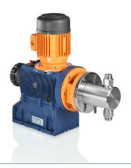
The plunger metering pump Sigma SBKa is an extremely robust plunger metering pump with high-performance plunger and the option to adjust the pump capacity in 0.2% increments. It offers a wide range of power end versions, such as three-phase or 1-phase AC motors, even for Exe and Exde areas with ATEX certification.
