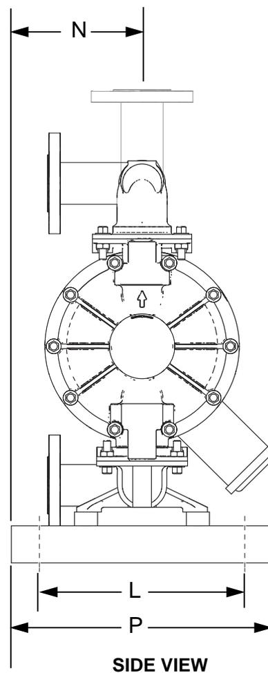
Dimensions B, C, F, G, H and M can vary by up to 1/4 in. (6.3 mm) depending on the seat and diaphragm material fitted in the pump.
