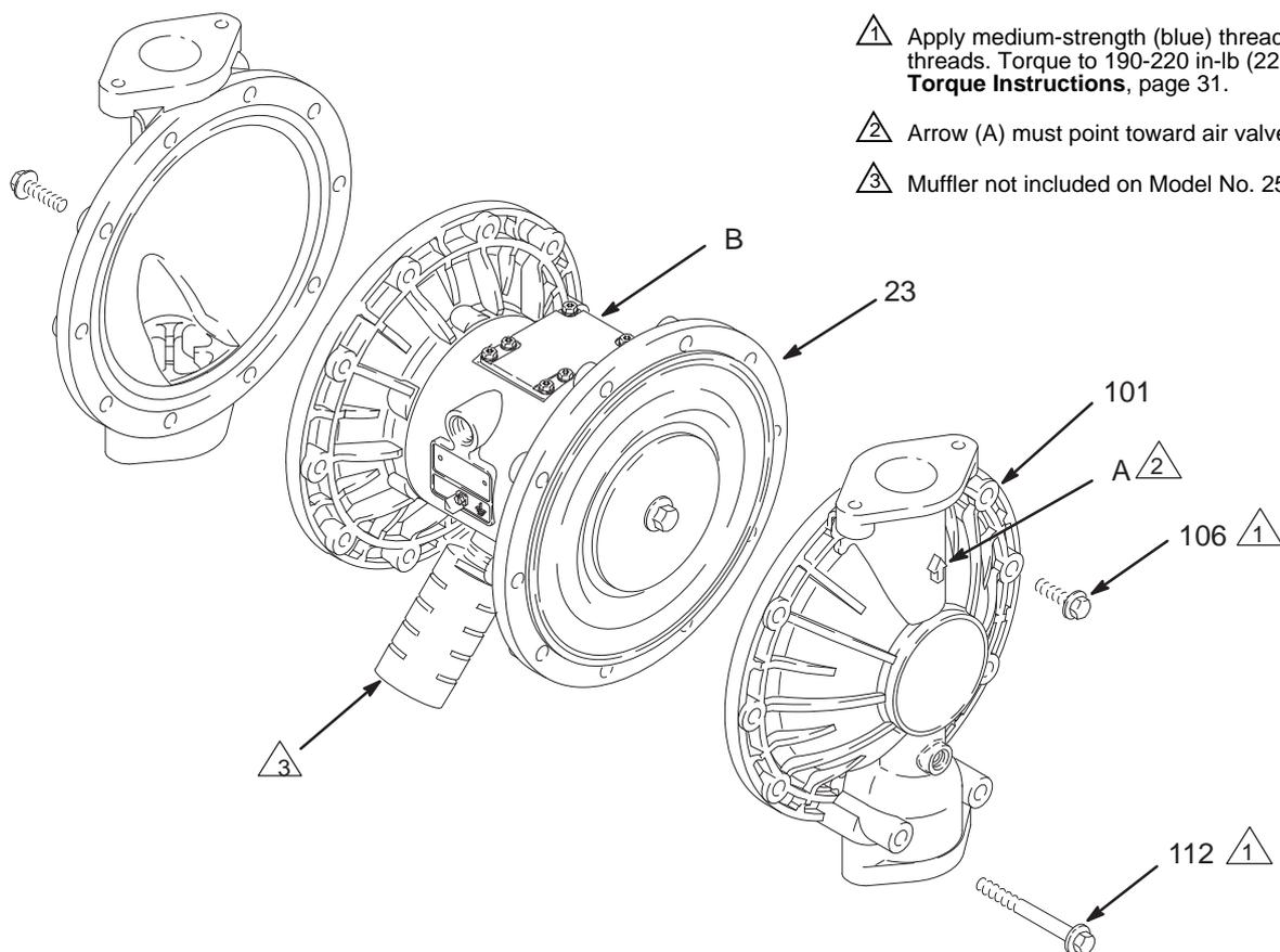
! Apply medium-strength (blue) thread locker to the threads. Torque to 190-220 in-lb (22-25 N•m). See **Torque Instructions**, page 31.
