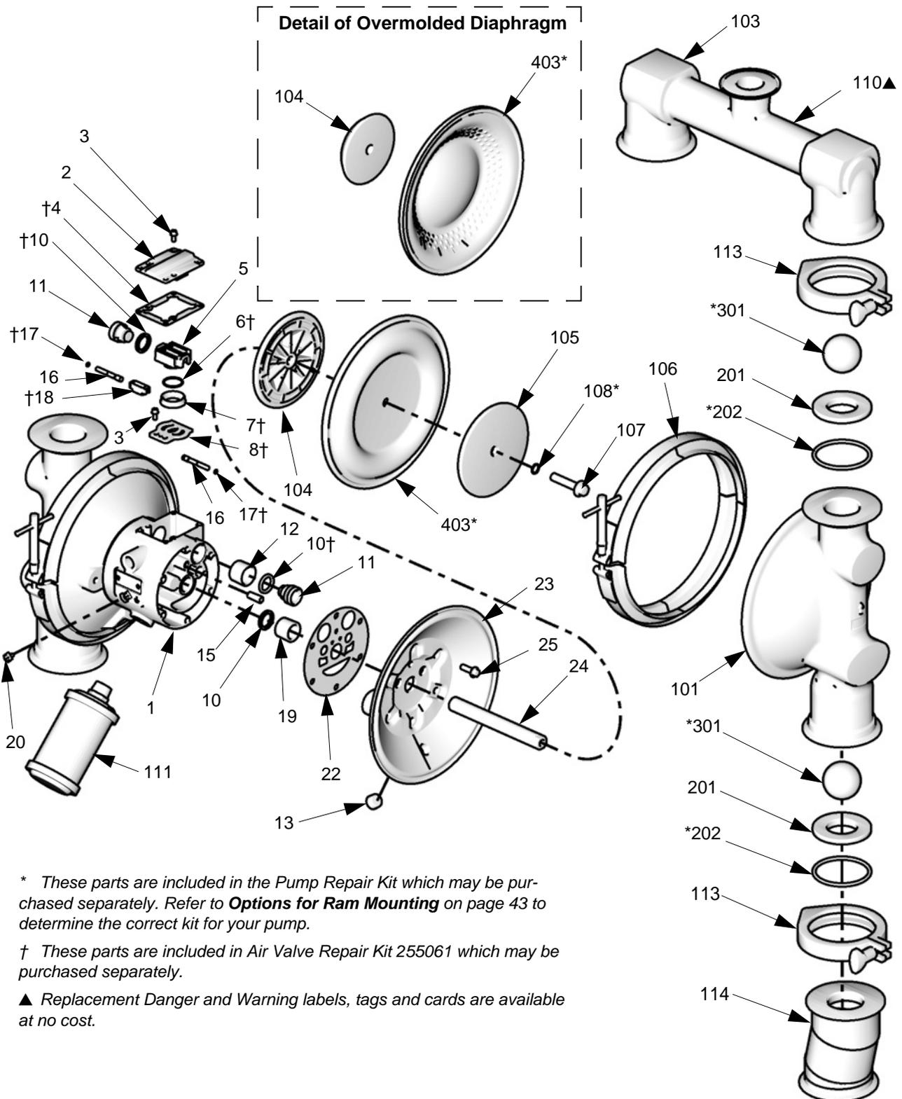
\* These parts are included in the Pump Repair Kit which may be purchased separately. Refer to **Options for Ram Mounting** on page 43 to determine the correct kit for your pump.
