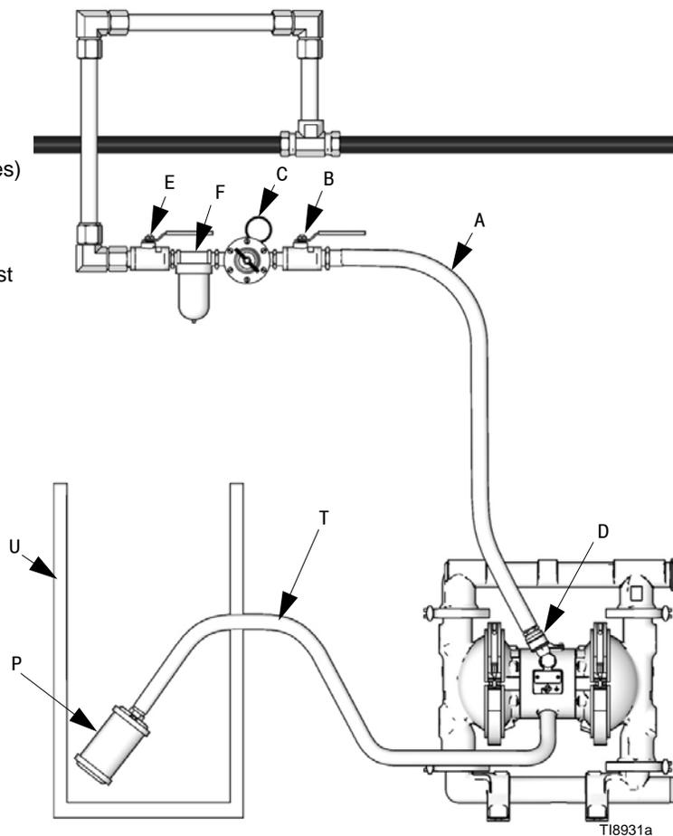
**FIG. 4 Venting Exhaust Air**
