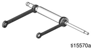
10. Remove the valve plate (108) and the piston (107). Remove the bearings (110) from the piston. (Model 24G761 has two bearings; Model 24G762 has three bearings.)
