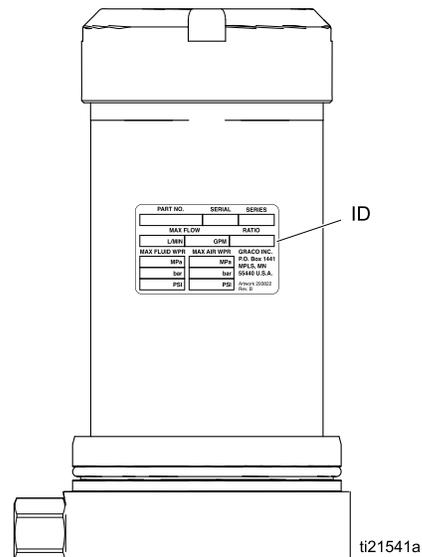
**Maximum Air Inlet Pressure: 100 psi (0.7 MPa, 6.9 bar)**
