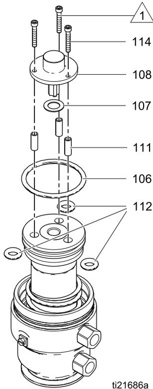
8. **Install assembled air valve from kit:** Lubricate and install new o-rings (106 and 115). Use pipe sealant on the threads of the valve (105) and torque to 15 to 20 ft-lb (20.3 to 27.1 N•m). Use a screwdriver as shown, if needed.
