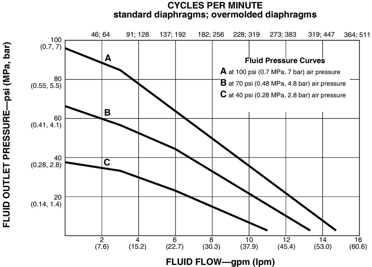
To find Fluid Outlet Pressure (psi/MPa/bar) at a specific fluid flow (gmp/lpm) and operating air pressure (psi/MPa/bar):
