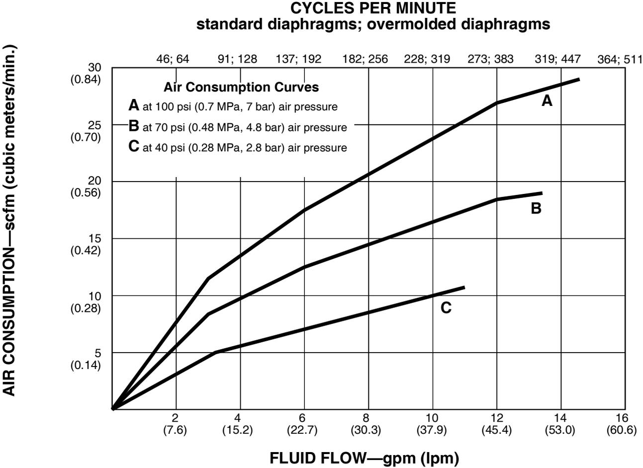
To find Pump Air Consumption (scfm or m<sup>3</sup>/min) at a specific fluid flow (gmp/lpm) and operating air pressure (psi/MPa/bar):
