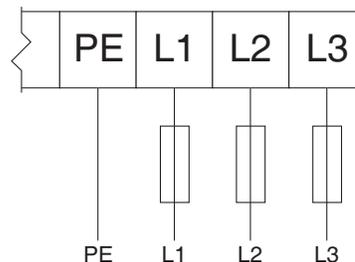
FIG. 4 190, 208-240 Vac 3 Phase Input/190, 208-240 Vac 3 Phase Output
