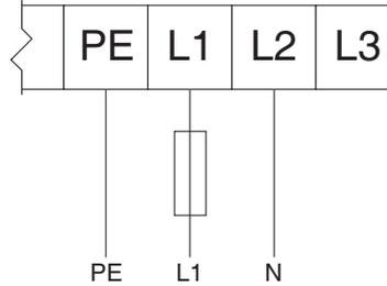
FIG. 3 208-240 Vac 1 Phase Input/208-240 Vac 3 Phase Output
