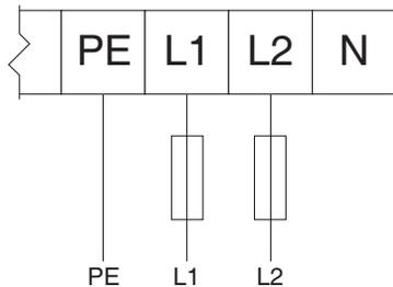
FIG. 2 240 Vac 1 Phase Input/240 Vac 3 Phase Output
