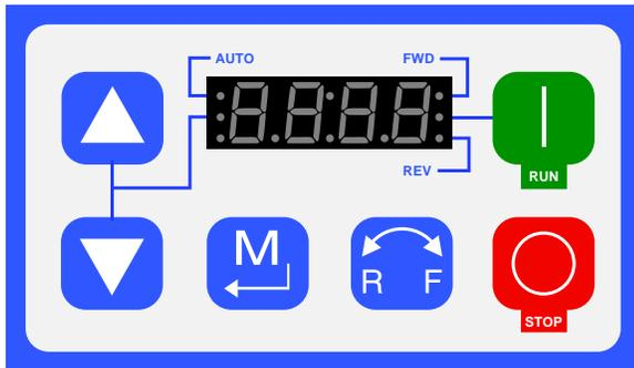
Figure 15 VFD Control Panel
