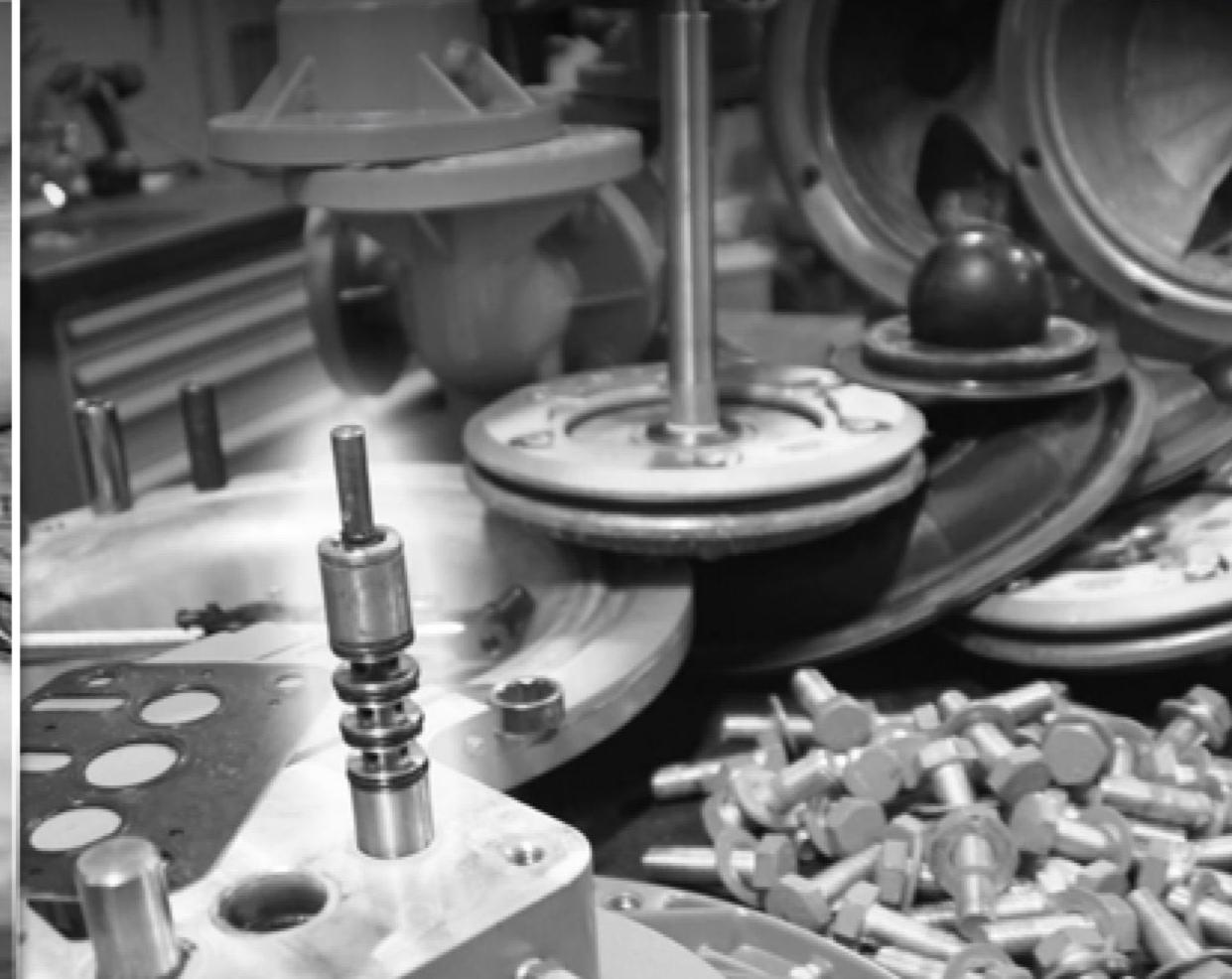
The Air Motor's Pilot Valve is the Most Often Serviced Part on an AODD Pump
