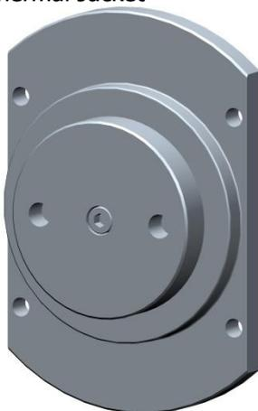
Figure 8 - End cover - thermal jacket
