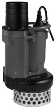
The KRS-series of energy-saving type is a submersible three-phase cast iron high volume heavy-duty drainage pump driven by a 4-pole motor. It consumes less energy than the standard KRS-series at lower head applications. The cast iron body, combined with the low speed motor, presents extra durability for use in the most demanding conditions. The top discharge, side flow design assures efficient motor cooling even when it operates with its motor exposed to air.
