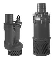
The KRS-series is a submersible three-phase cast iron high volume heavy-duty drainage pump driven by a 4-pole motor. The cast iron body, combined with the low speed motor, presents extra durability for use in the most demanding conditions. The top discharge, side flow design assures efficient motor cooling even when it operates with its motor exposed to air.\*
