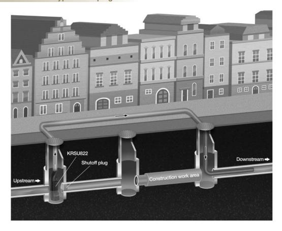
Since sewage piping suffers from aging-related deterioration and can be damaged by earthquakes, sewage piping requires repairs and replacing at regular intervals. In sewage piping repair work, consideration should be given to area residents inconvenienced by the repair work, and additionally to work efficiency and the safety and health of workers who handle inflow sewage. For this purpose, provisional draining that temporarily bypasses sewage via a pump is extremely effective.
