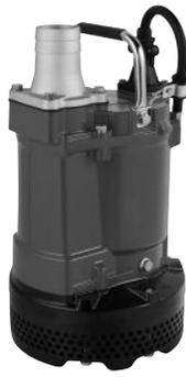
The KTV-series is a submersible three-phase portable drainage pump. The pump body is made of die-casted aluminium alloy, which is extremely advantageous in terms of portability. The sleeves that protect the pump casing, oil casing and water passages are made of synthetic rubber as a consideration against wear. The top discharge, side flow design assures efficient motor cooling even when it operates with its motor exposed to air. The slim design allows the pump to be placed in a confined space.
