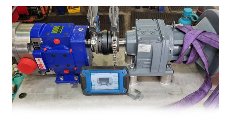
Shaft misalignment is responsible for up to 50% of all costs related to rotating machinery breakdowns. Reduce these breakdowns, production losses, high energy consumption, overheating, excessive vibration, and premature wear and tear with our laser alignment services.
