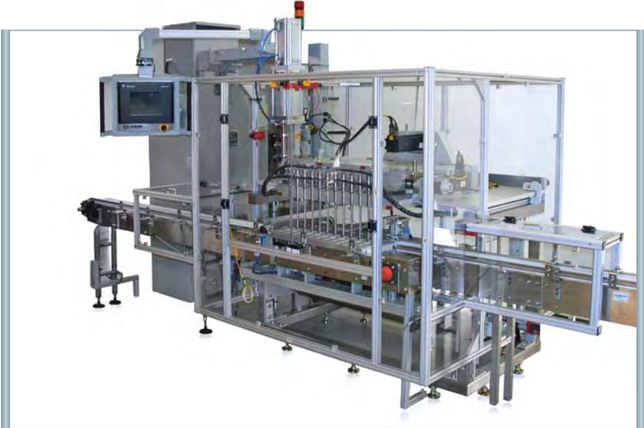
**HIBAR'S IN-LINE INTERMITTENT MOTION FILLING SYSTEMS** are designed to provide both economy and flexibility for customers with a diverse product range. An indexing system is used to transport containers in groups through the fill area. Quick change parts are available to accommodate product change-overs in minutes.
