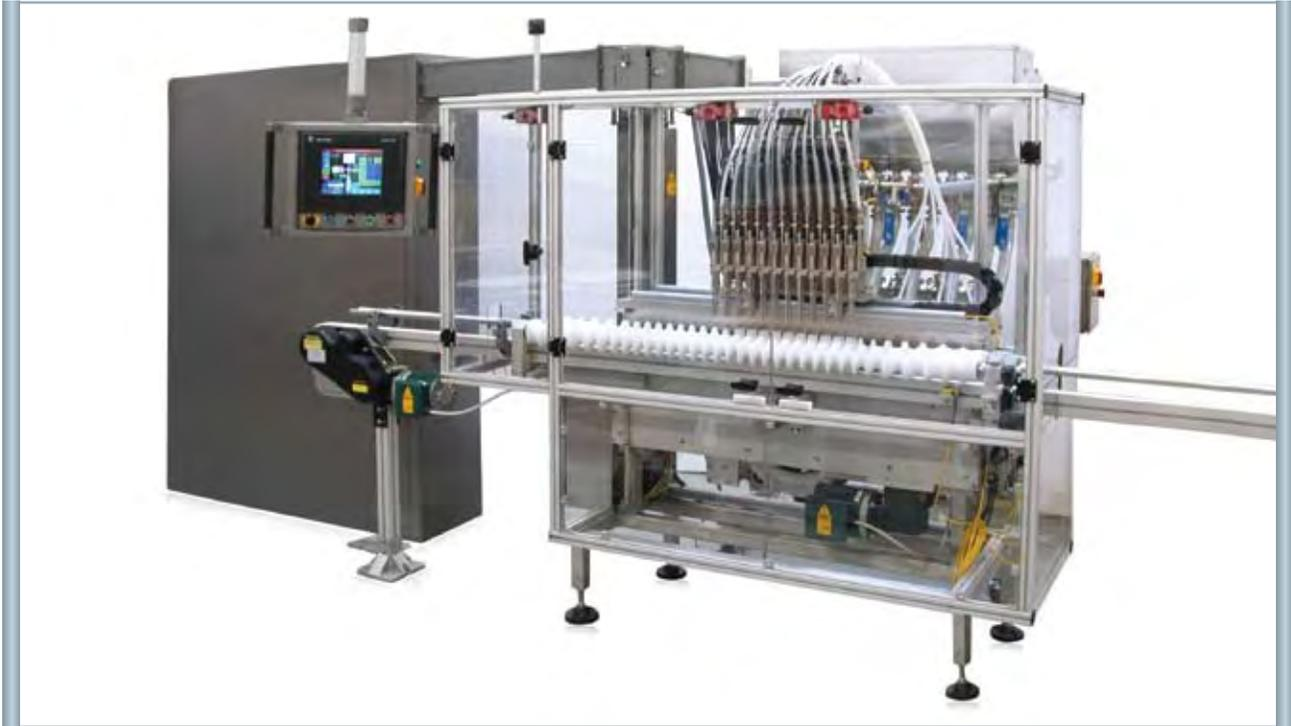
**HIBAR'S IN-LINE CONTINUOUS MOTION FILLING SYSTEMS** are designed with performance and versatility in mind. The compact "Walking Beam" design, together with our innovative dual screw bottle feeding is capable of filling bottles at rates up to 300 bottles/min. With one simple adjustment, the integrated "Universal" dual screw system is able to handle a wide range of bottle sizes with no change parts required.
