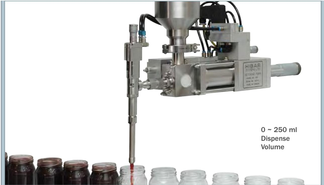
The **NEW HIBAR 4H SERIES ROTARY VALVE STYLE DISPENSING PUMPS** are ideally suited for higher viscosity applications in food, cosmetic, technical and pharmaceutical industries. Liquids with up to 100,000 cps viscosities and including particulates are easily handled with our durable ceramic rotary valve design. Dispensing accuracies of  $\pm 1/2\%$  or better with positive cut-off and no drip can be easily maintained without readjustment or recalibration.
