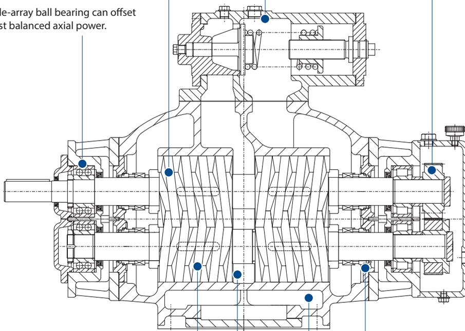
Separate construction between shaft and screw allows for a choice of materials for each.
