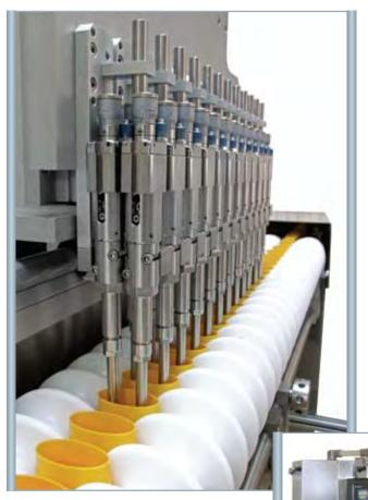
Heated Filling Systems are available, utilizing sealed heated chambers or electronic cartridge heaters.
