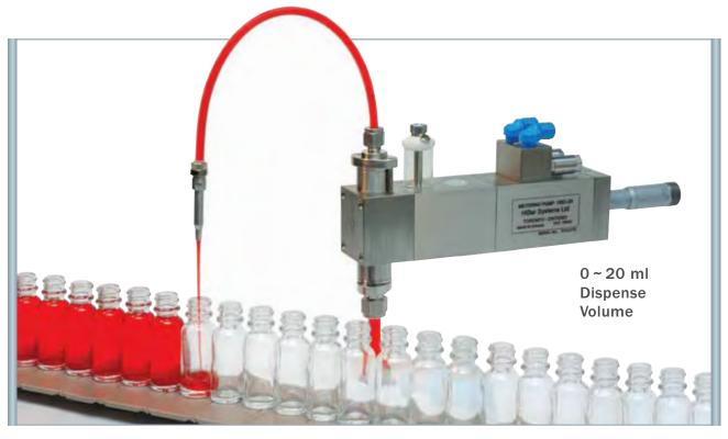
The **HIBAR B SERIES CHECK VALVE** style Dispensing Pumps have proven reliability having serviced the cosmetic, food, pharmaceutical and technical industries for over 30 years. These pumps are ideally suited for low to medium viscosity applications (<2000 cps) that require dispensing of .020 ml to 20 ml per shot.
