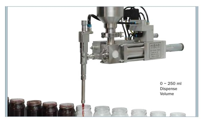
The **NEW HIBAR 4H SERIES ROTARY VALVE STYLE DISPENSING PUMPS** are ideally suited for higher viscosity applications in food, cosmetic, technical and pharmaceutical industries. Liquids with up to 100,000 cps viscosities and including particulates are easily handled with our durable ceramic rotary valve design. Dispensing accuracies of  $\pm 1/2\%$  or better with positive cut-off and no drip can be easily maintained without readjustment or recalibration.
