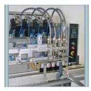
High Viscosity Make-up Filler with Star Wheel Indexing System
