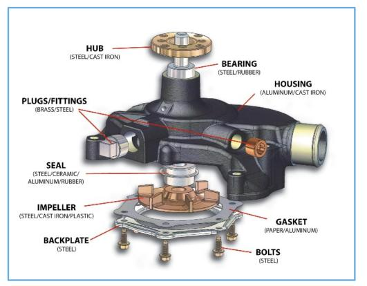
Centrifugal Water Pump Components
