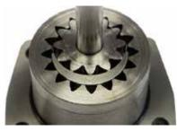
Internal gear pump
