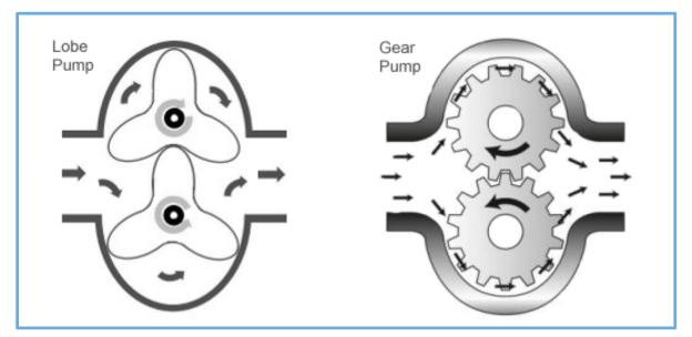
Positive Displacement Water Pump Components
