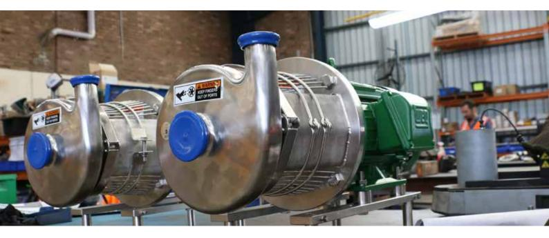
Pumps have strict tolerances and precise conditions under which they must operate to generate the Best Efficiency Point or BEP. Every pump has a chart showing the performance curves and how to attain the BEP. Pump manufacturers calculate performance curves with a pressure gauge and a flow meter connected to the discharge port to find the optimal configurations of piping, type of fluid and head. The discharge capacity can be calculated for any head.
