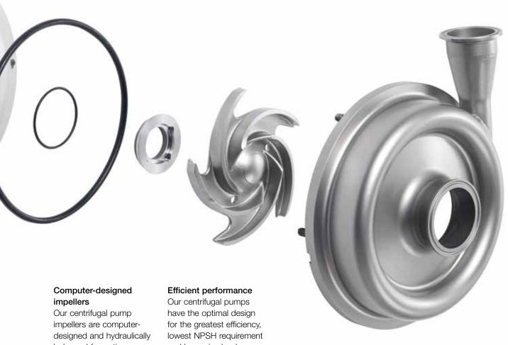
Our centrifugal pump impellers are computer-designed and hydraulically balanced for optimum performance. Both the impellers and their retaining screws (optional) are smooth, which keeps them from accumulating product and makes cleaning more effective.
