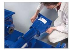
5. Turn the feed chamber and rotor and stator into position and secure
