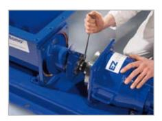
6. Unscrew the rotor from the stator
