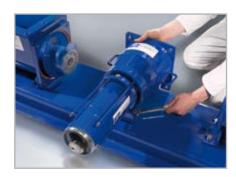
8. Remove the stator
