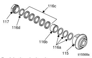
Fig. 6. Intake valve housing
