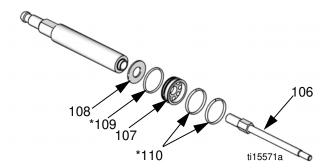
Fig. 4. Remove piston and seals
