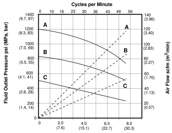
Fluid Flow gpm (lpm) tested in No. 10 weight oil
