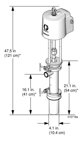
$^{\star}$  Add 4.7 in. (12 cm) to allow for full extension of the priming piston rod.
