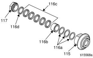
Fig. 3. Intake valve housing
