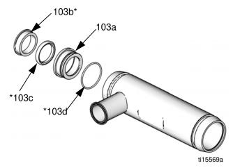
Fig. 5. Remove u-cup seal assembly
