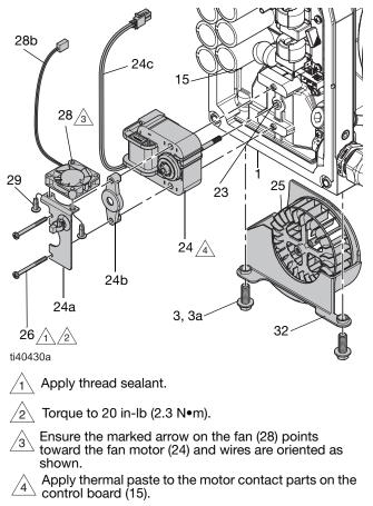
FIG. 9: Reassemble the Fan Assembly
