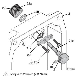
FIG. 10: Control Knob Assembly
