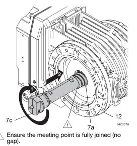
FIG. 17: Insert Rotor Greasing Tool
