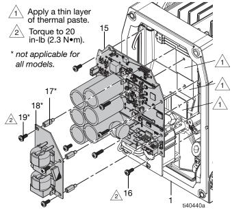
FIG. 11: Control Board and Filter Board
