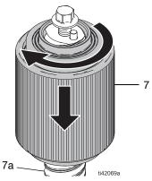
FIG. 16: Assemble the Shaft and Rotor
