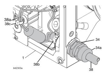
FIG. 4: Power Cord/Cable (F-2 and F-4 motors)
