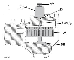
Apply thermal paste to the contact surface between the fan motor (24) and stator housing (1).
