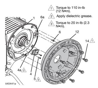
FIG. 12: Motor Sensor
