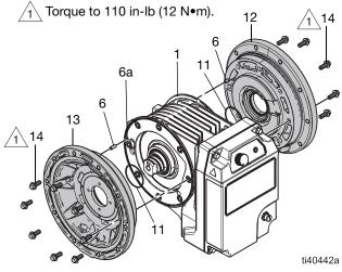
FIG. 13: Center Section, Load-side
