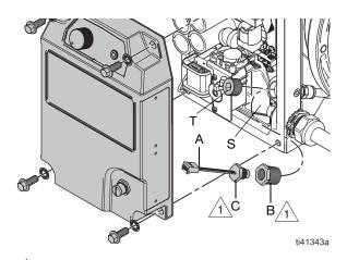
Apply Loctite 425 Assure<sup>™</sup> thread sealant to the threads.
