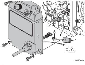
Apply Loctite 425 Assure<sup>™</sup> thread sealant to the threads.
