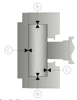
Figure 31 - Shim / clearance measuring
