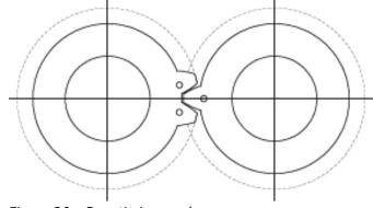
Figure 36 - Gear timing marks
