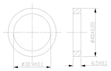
Figure 26 - L Cup insertion tool
