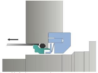
Figure 20- Seal seat removal
