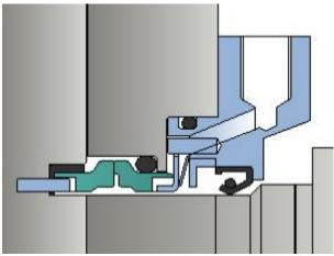
Figure 10 - Flushed single seal (Size 4-8)
