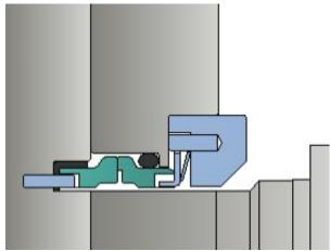
Figure 9 - Single mechanical seal (Size 4-8)
