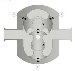
Figure 29 - clearance measuring
