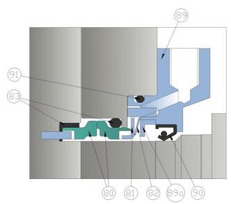
HP & LH Flushed Mechanical Seal
