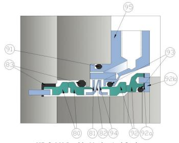
**HP & LH** Double Mechanical Seal
