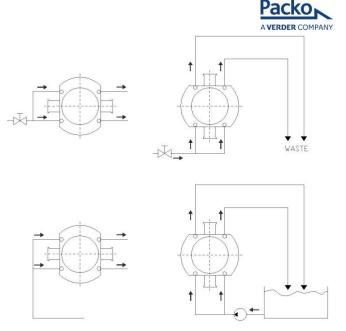
Figure 11 - Suggested low pressure flushing system
