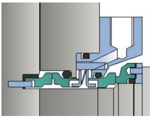
Figure 12 - Double mechanical seal (Size 4-8)
