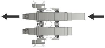
Figure 33 - Removing shafts
