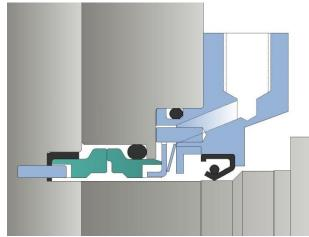
Figure 27 - Single flushed mechanical seal
