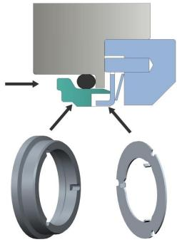
Figure 24 - Fitting stationary seat
