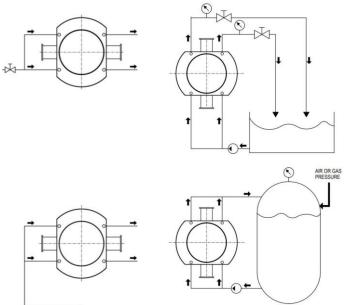
Figure 13 - High pressure liquid supply for double seals
