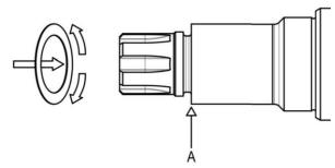
Figure 32 - Fitting shims
