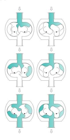
Figure 1 - Principle of operation (Showing vertical mounting)
