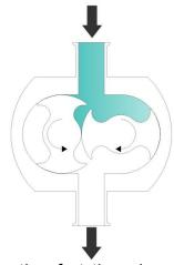
Figure 16 - Direction of rotation - viewed from pump head (Principle applies to all mounting orientations)
