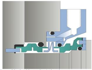
Figure 28 - Double mechanical seal
