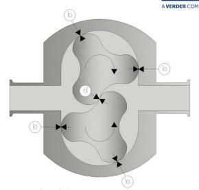
Figure 30 - Shim / clearance measuring
