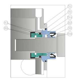
**HP 3 Size** Flushed Mechanical Seal
