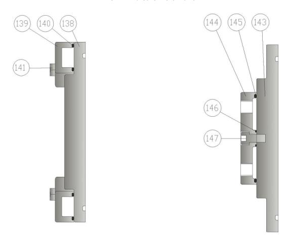
**HP & LH** Thermal Jacket – Pump Head
