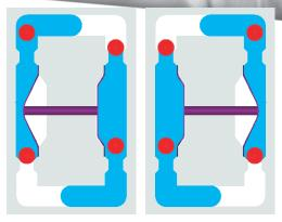
end of the stroke is reached, it reverses automatically and the cycle is repeated in the opposite direction. In the second figure, liquid is drawn in by the left-hand diaphragm and displaced by the right-hand diaphragm. The liquid is displaced – and thus conveyed – by the compressed air. The diaphragms merely serve as barriers and are not pressurized. This is a fact of decisive importance for the service life of the diaphragms.
