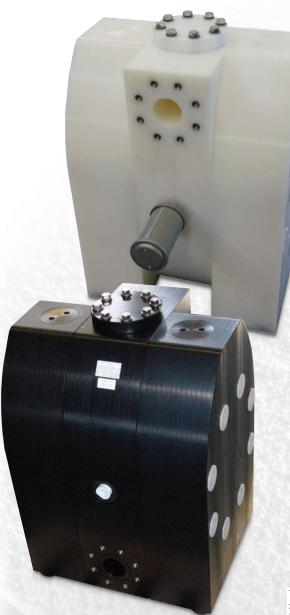
The pump size E 80 extends the E-Series range to seven sizes. With a maximum capacity of 48 m³/h the E 80 is proper for an efficient circulation of great quantities. Housing material is PE or PE conductive. The housing bolts are not tighten against a ring. The using of spring washers allows a high security and less leakage liability.
