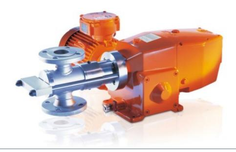
The plunger metering pump ORLITA DR does not need valves and can therefore be operated within a broad stroke rate range. It is therefore suitable for use with high-viscosity and extremely high-viscosity media of up to 10<sup>6</sup> mPas within a wide temperature range of -40 °C to 400 °C.
